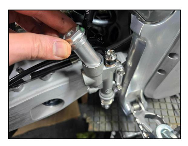
4. Insert the junction valve and screw my hand, you will feel tension as the junction valve compresses around the o-ring, once to the base torque to 20nm
