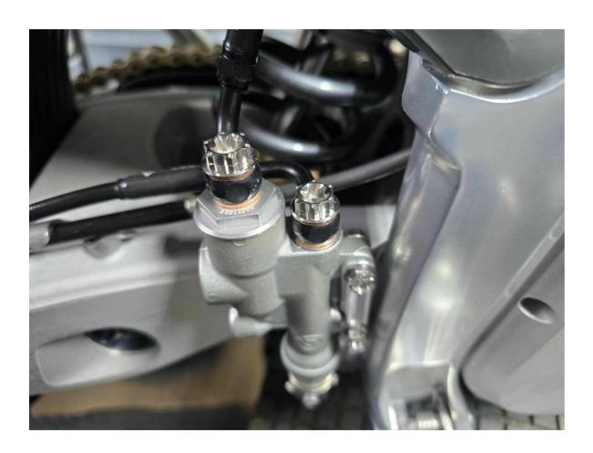
5. thumb brake or lever brake then mounts into the junction valve as shown which is an M10x1.00 thread.
