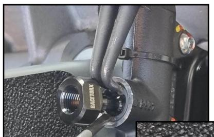
6. Using small circlip pliers install the circlip, it may help to use a small flat head screw driver on the opposite side to install level. Inspect the fit to ensure that the circlip is seated under the lip properly.
