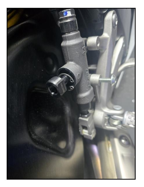
5. Press junction valve into master cylinder.
