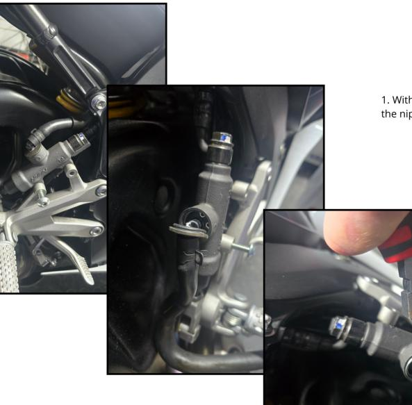
1. With circlip pliers, remove the circlip and pull out the nipple.
