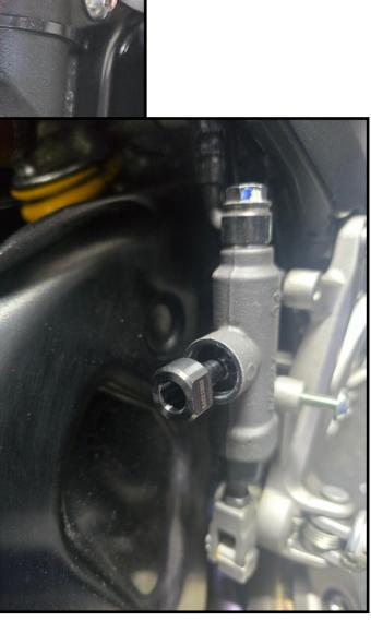
6. Using small circlip pliers install the circlip, it may help to use a small flat head screwdriver on the opposite side to install level. Inspect the fit to ensure that the circlip is seated in the circlip groove.
