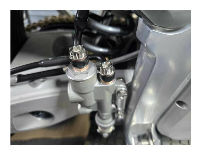
4. thumb brake or lever brake then mounts into the junction valve as shown.
