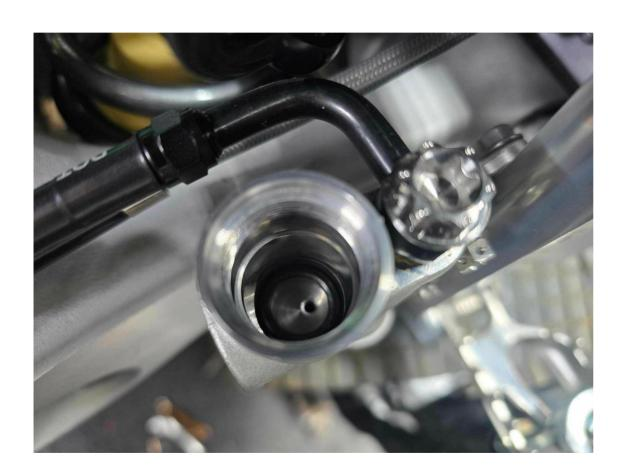
1. Remove the screw cap and O-ring.
