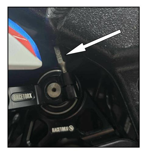
7. A stubby allen key or similar will be required to tighten the allen pinch bolt due to the tight space.10nm is the correct torque settings for the pinch bolt.
