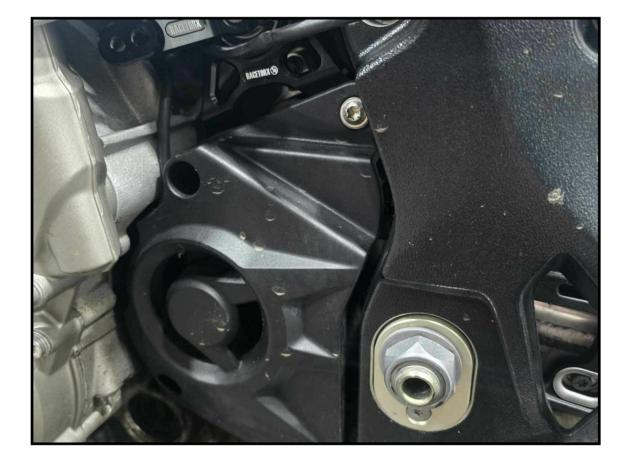
8. Fit sprocket cover over the bottom plastic spacer included and over the gear shift support.
