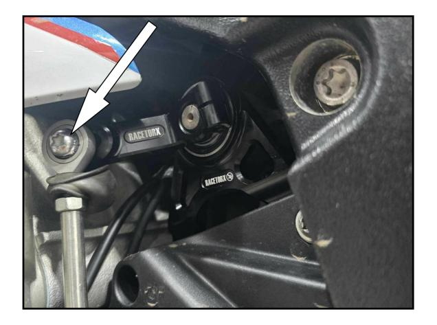
10. Fit bolt and torque to 10.7NM and be sure to re-fit quick shifter plug and then place rubber cover back over the bolt.
