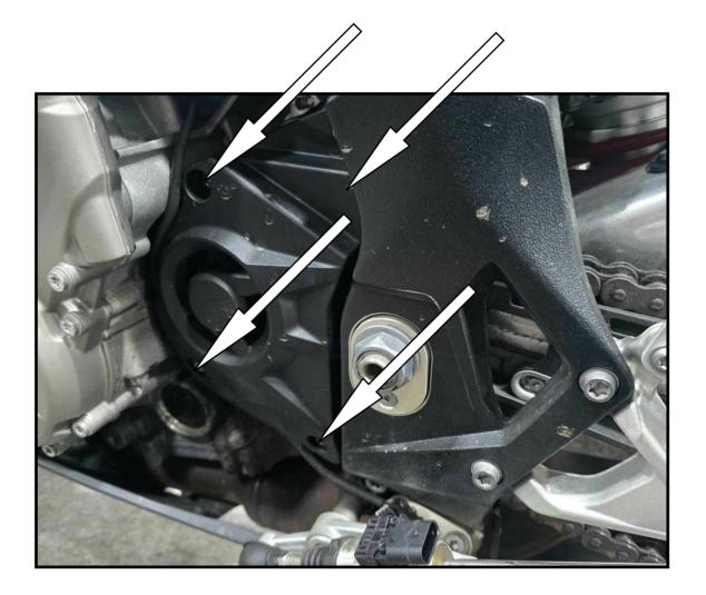
3. Remove bolts holding sprocket cover, removing sprocket cover make sure the 4 spacers in the cover are present and not to lose them as they are not pressed.
