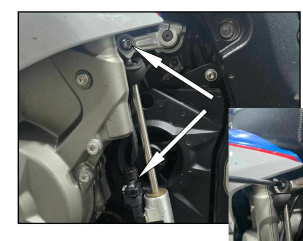
1. Start by removing the bolt and plug on the quick shifter.
