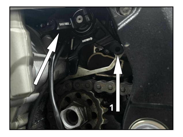
5. Slide the assembly over the gear shaft at the same orientation as the OEM arm.
