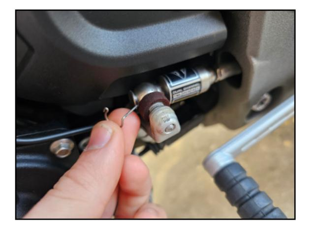
2. Remove retaining pin from the Quick shifter & keep safe.
