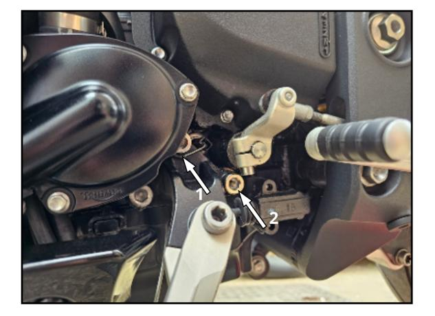
1. To begin, remove/replace bolts 1 & 2 with supplied titanium M10 bolts with washers.
