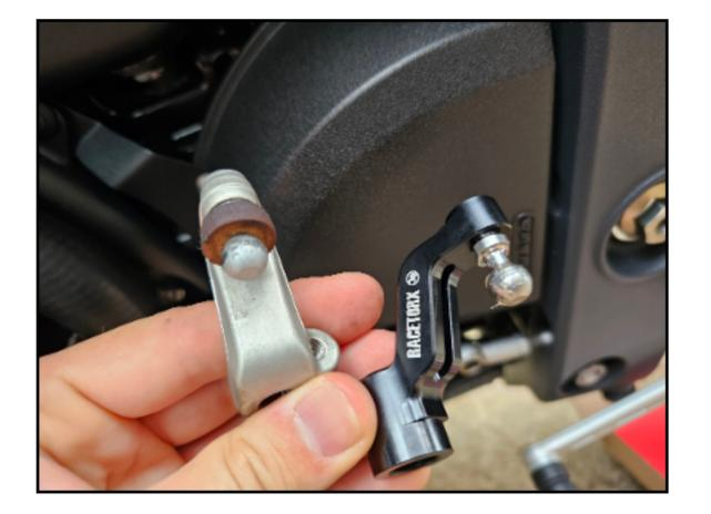
8. Mount titanium ball joint & torque to 10NM
