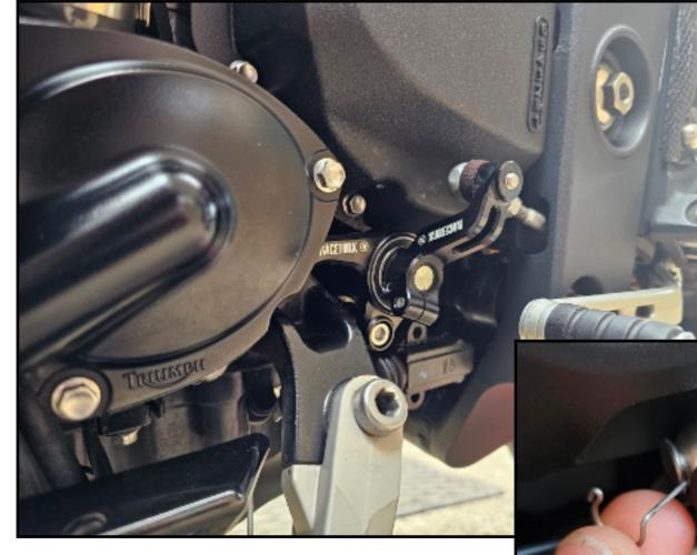
10. Pull the quick shifter head onto the Titanium ball joint and refit the retainer clip.
