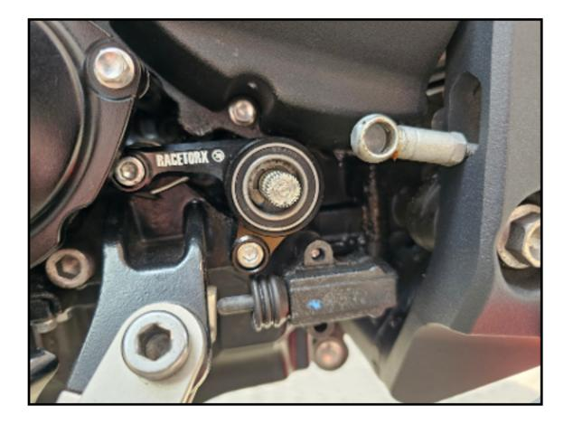
7. loosely mount the gear shift support frame with supplied M6x20 bolts
