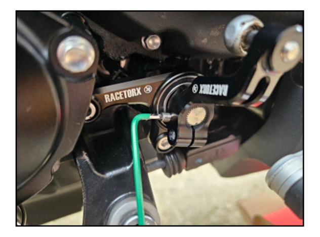
9. Slide the Racetorx gear arm onto the spline and through the bearing gently & in the correct orientation as per OEM .
